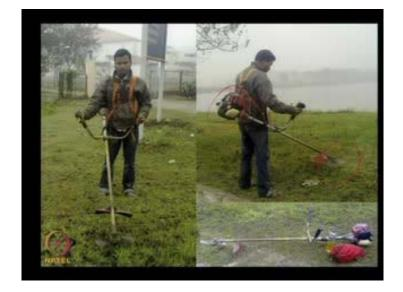
In this case, the blade is moving automatically, but while holding it a static load is coming on the shoulder, because is a constant holding like this and in a to keep in a specific spacing, though the harness and etcetera are already designed, but still it imposes some problem so how further development can be done.
