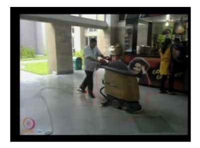
Here the equipment - the work equipment - it moves by self, but the controlling has to be done by person. And while controlling it says, now what are the postures they are feeling, and when it is being used, this floor becomes very slippery; what would be the wearing - foot wearing matter - where so that the person should not slip off on the floor.
