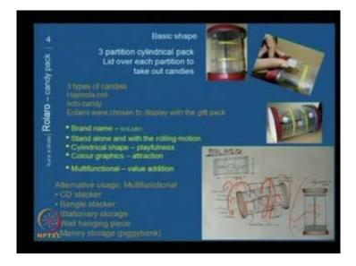
Number fourth is that rolaro candy pack is the name given to this package. The basic shape is a drum type of thing where the 3 partition cylinder pack lid from the both sides
