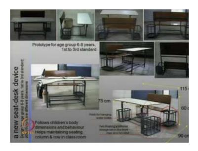
The final design developed was like this. In this final design, the seat plate, backrest, 5 degree inward inclined tabletop, the gap and this is that fixed books holder and this is a
