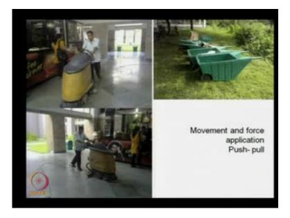
So, the design should go along with the normal body access movement. Now, movement and force application push - pull this type of products either needs to be pulled or pushed; this type of product it requires mostly the pushing force with the mechanical and electrical assistances.
