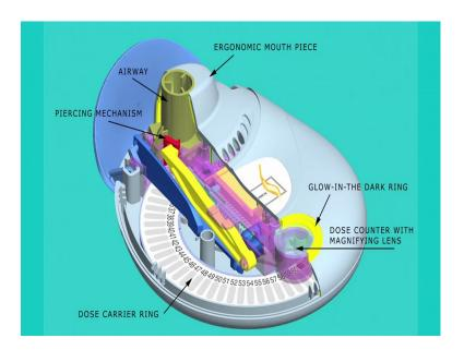
The inner-inhaler has a very resourceful design and it is designed to increase efficacy by helping the drug reach deep in the lungs where it is most required and give faster relief to
