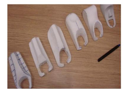
And the whole design now has to go back to the drawing board go back to conception. Again make three concepts and come back to the production because you are not lost much, because you just made one prototype. How can this vein tracer be more easy to hold, how can it be smaller, multiple thermocol mockups, same process we will go out in the field, check out with care givers check out with nurses, check out in the hospitals. Which form will work, which is convenient to hold?
