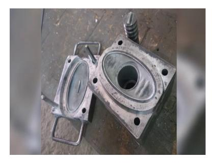
The two three processes of molding, so, this is compression molding, where we did compression molding of the neoprene rubber. And you can see the tool parts. So, we made this tools very quickly with the tool manufacturer and we got the components out.
