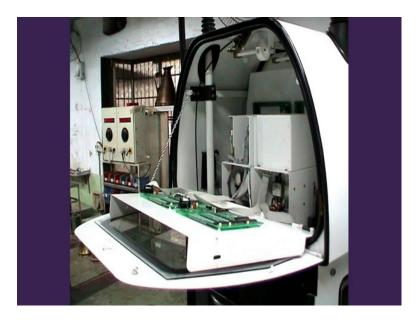
This whole panel drops down like this there the petrol pump lifted like this here we are dropping down like this. So, you need to have all the features inside the pump without that maintenance features it does not work. So, maintenance is very easy.
