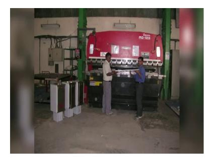
And you can take it for fabrication where you get flat sheets; you take the flat sheets to this machine to do the bending. What is a very interesting about CNC bending operation is that this bending operation is very very intricate and very accurate.
