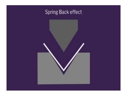
Stainless steel has a property of spring back. If you bend 90 degrees, finally you land up with some 87 or 86. So, this machine has the capability a computer to calculate the material properties of stainless steel, you can feed in the grades with 304 and it will bend exactly 90 degrees.
