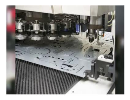
So, and then they also took us to their manufacturing unit, which is called the Jindal Architecture, where we produced the components using CNC punching. What is the advantage of computer numerical punching of a sheet before you fold it?
