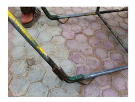
They weld them together and we also get know from metallurgy that when you weld galvanized iron pipes together the welding is not very strong the metallurgy point of view. Because constant loading and cyclic loading there is cracking in the welded joints and then also it is very very heavy.
