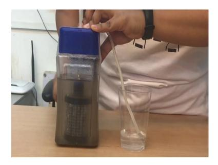
So, we immediately went online, we purchased this pump, fitted to a rig, see the rig is very critical this is a working rig there is a bottle of dirty water there is a pump which is what we are using and then we have the filter which is giving us all the filtration. You think I can go and give this to CRPF jawans?
