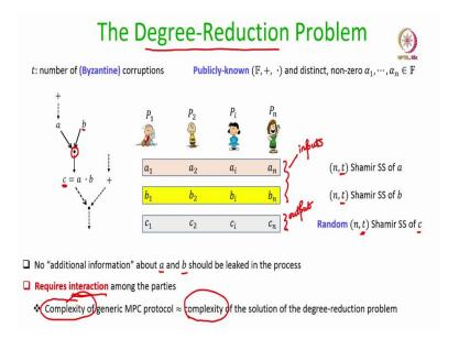
So, this degree reduction problem occurs in the context of shared circuit evaluation in the BGW protocol. The problem is the following. Suppose you are given a circuit where we have a multiplication gate in the circuit such that the inputs of this multiplication gate, they are secret shared as per an instance of Shamir secret sharing, where the degree of the sharing is t, with each party holding its respective shares.
