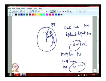
Let us say this is a disk, you have a block here and you want to move to the block. So, this could be on one track this could be another track; that means, that I have to first move from this track to this track, so that is the track seek time, followed by I have to move my head from here to it was somewhere here right and it has to move this much this distance. So, there is also here rotational aspect.
