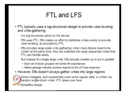
Now, let us look at the interaction between FTL and LFS it turns out FTL itself uses a log structured design. So, now, we have a flash friendly file system using LFS and we have the FTL typically if we see the design of the FTL itself what is FTL this is the translational layer it turns out the flash translational layer itself uses a log structured design because it its used to provide wear leveling and write gathering because that way also it has to write in larger chunks at the lower level.
