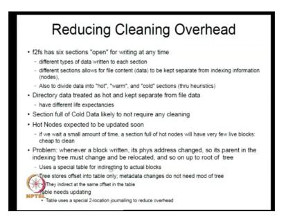
So, as I mentioned earlier this f 2 fs has six sections open for writing at any time different types of data written to each section different section allows for file content to
