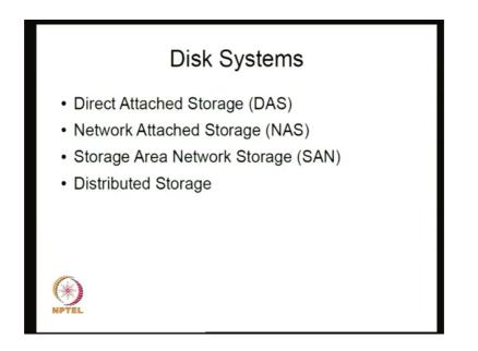
I think in disk systems there are varieties of them you can see one is called the direct attached storage, what is this? This is a typical pc kind of situation in a pc you have a disk attached to the bus pc bus pci bus and this bus called direct attached storage that. Of course, in larger systems, you will have many more disks attached to the same bus.
