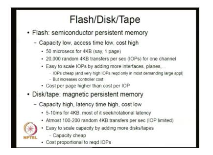
Now, now we already seen three types of technologies flash disk and tape. Flash is semiconductor persistent memory, what is a capacity what is it characteristics? Its capacity is low compared to disk for example, an access time is low compared to disk cost is high compared to disk. If you look at a disk or tape it is a magnetic persistent memory, capacity is very high compared to flash, here we talked about access time here we talk about latency time because it can involve seeking also ok.
