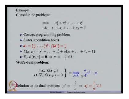
So, we have a problem to minimize norm x square subject to the constraint that x 1 plus x 2 up to x n equal to 1. This is a convex programming problem because the objective function is convex the constraint set it is affine. So, Slater's conditions are automatically satisfied. Now, we can see that the solution to the this problem is that all values of the coordinates are same and they are 1 by n. And, they are optimal objective function value is 1 by n.
