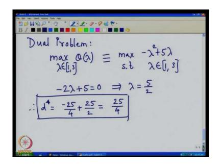
The dual problem is maximize theta lambda with respect to lambda which is in the interval 1 to 3, and this nothing but maximize minus lambda square plus 5 lambda; subject to lambda belongs to 1 to 3. Now, this is a concave function. So, again we differentiate this function with respect to lambda equate it to 0. And, what we get is minus 2 lambda plus 5 equal to 0 and which gives lambda is equal to 5 by 2.
