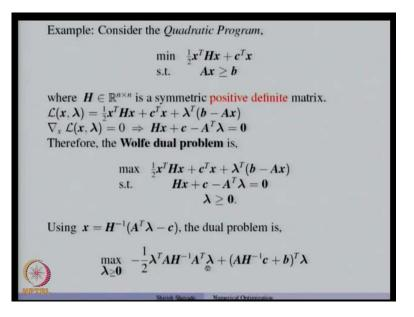
So, let us see how to do that? So, as in the previous case we write the Lagrangian and then said that the gradient of the Lagrangian with respect to x to 0; which gives us this equation H x plus c minus a transpose lambda equal to 0.
