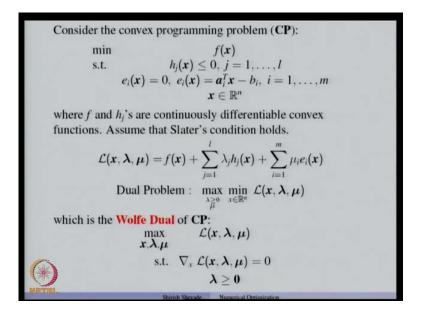
So, let us consider a convex programming problem; where f is a convex function. The objective function is convex the constraint the inequality constraints are h j (x) less than or equal to 0. And, the function h j (x) corresponding to these inequality constraints is also a convex function; the equality constraints are given by a i transpose x minus b i equal to 0. And, let us consider the set x to be entire set r n.
