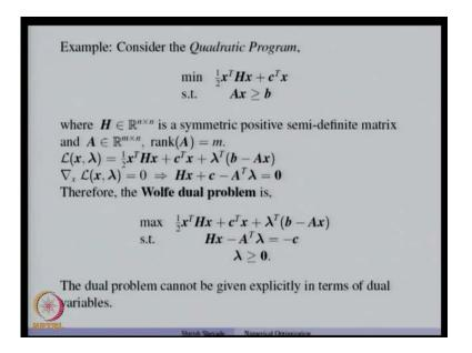
Let us consider a simple example. Let us consider a quadratic program to minimize x transpose H x plus c transpose x subject to the constraint that Ax equal to b. Now, the H matrix is a n by n positive symmetric semi definite matrix and A is n by m matrix and the rank of A is m. Now, we assume that the Slater is constraint qualification holds; this is a convex programming problem. So, we can write the Lagrangian as the objective function
