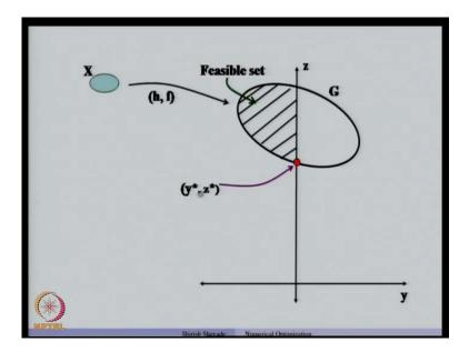
So now, the shaded portion of the set G is the feasible set, because that satisfies y less than or equal to 0. Now, among all this points, which are feasible than to find out the point, which has the least ordinate and that point is this point. So, let the coordinates of this point be y star, z star.
