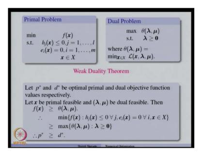
Now, now let us look at the weak duality theorem, which states that, if p star and d star are optimal primal and dual objective function values then p star is greater than or equal to d star. This is a straight forward extension of the previous theorem, that we saw, note that, if x star is solution to this primal problem and lambda star, mu star is dual is a solution to this dual problem. Then p star is nothing but f of x star and d star is nothing but theta of lambda star, mu star.
