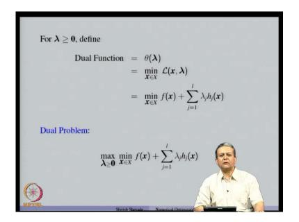
And similarly, one can define a dual function, which is theta lambda and that is nothing but minimum of the Lagrangian function, and then the idea is to maximize this theta lambda. So, maximize with respect to lambda the minimum of the Lagrangian function with respect to x. So, you will see that, the dual problem is the max min problem, max min of the Lagrangian and primal problem is the min max of the Lagrangian. And in this discussion, we have used Lagrangian function as a payoff function.
