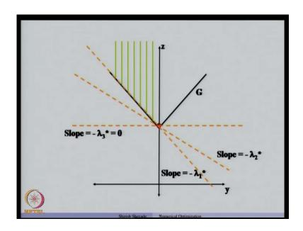
Now, let us see some examples, so the first example that, we are going to see is one here. So, the set G is the set of all points above this function and out of those possible points, the set of feasible points is marked here, so these are the points, where y is less than or equal to 0. And what we are interested in finding out, the minimum the minimum z such that, y less than or equal to 0. And therefore, clearly this is the optimal primal objective function.
