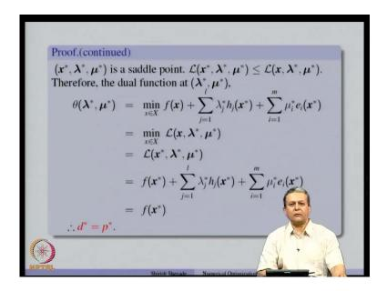
So now, we can show that, the duality gap does not exist under the Lagrangian saddle point condition. So, the first thing that, we showed was that x star is a primal feasible that is, x star less than or equal to 0 e i (x star) equal to 0. For all I, we are given that x star belongs to the set x and we also showed that the complimentary slackness condition, which we studied, when we studied k k t conditions, that also holds. That is, lambda j star h j (x star) equal to 0.
