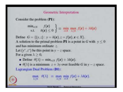
So therefore, what we are interested in solving max of theta lambda, where lambda is a non negative quantity and max of theta lambda is nothing but max of min of the Lagrangian. So now, you will see the dual relationship between the two problems, so this is our primal problem and this is our dual problem. The primal problem is the min max of the Lagrangian, the dual problem is the max min of the Lagrangian.
