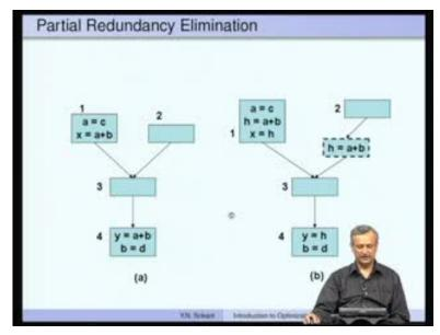
Next, optimization is a very important one called the partial redundancy elimination. There are actually, you know many optimizations which this particular PRE as it is called subsumes. For example, loop invariant code motion gets subsumed in this. If we do this properly, then 2 or 3 types of common sub expression elimination can also gets subsumed by this; so 2 or 3 optimizations can all be subsumed by this particular optimization itself.
