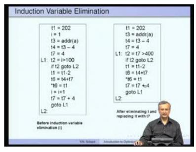
The next example is that of induction variable elimination, again the previous example we carry forward. So, before the induction variable elimination, let us say i is the induction variable we want to eliminate. Why is i called an induction variable? You see
