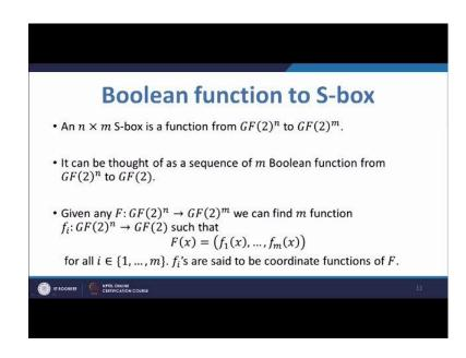
Now, the question is how we connect Boolean functions to S-boxes, the answer is in the slide. Suppose, I have got an n by m S-box, so that S-box is taking n bit input and giving me m bit output. So, I can consider that S-box has a function from GF 2 to the power n to GF 2 to the power m. So, to say each coordinate functions, let me draw it over here.
