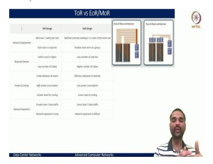
So, if we consider in terms of how these would compare, if we think of network deployment, in the ToR design, you need one switch per rack as an additional entity while in the end of the rack design, all the switches centrally reside in 1 to 2 racks of the same row that means you only have the aggregation switches that are being placed in one row. And you have eliminated the need for one switch per rack.
