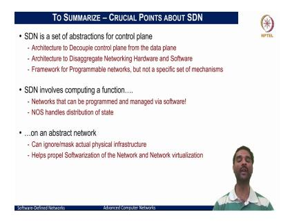
To summarize, SDN can be thought of as a set of abstractions for the control plane. In that, we began with SDN as an architecture to decouple the control plane from the data plane of the networking elements. Then we went ahead and showed that this architecture would also help disaggregate the networking hardware and software, enabling us to mix and match open hardware and proprietary software and vice versa to be run as networking elements.
