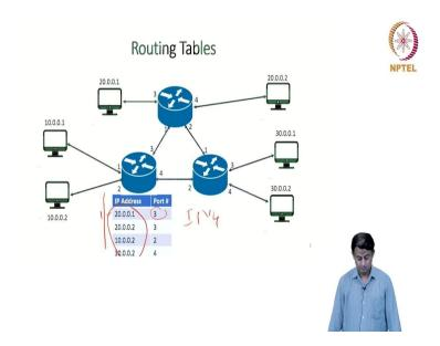
So, we saw last time the diagram similar to this. So, what you see here are a bunch of computers and three routers, and we see that the IP address table or the routing table in the router looks something like this. So, this is a simplified version of the routing table what you have is a bunch of IP addresses, so this is the IP address number 1; if you receive a packet with this destination IP address, you need to send it to this port number that is the meaning of that.
