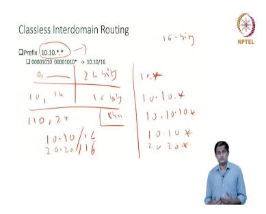
So, that brings us to the concept of something called prefix-based routing. So in effect, what we said is, if I am saying that my network address is 16 bits, the routing table entries are 16 bits. So, if it starts with 10.10. And then what I can do is I can denote that or the entries inside the routing table using this prefix notation 10.10.\* is actually a prefix notation.
