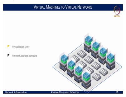
Let us try to understand about Network Virtualization in a bit more detailed fashion. The slide here with the picture shows exactly the composition of a typical enterprise network or a campus network, or even it could be mapped to a small-scale data center where we have the physical compute devices and storage devices and also the network elements like the switches and routers that connect these compute and storage elements.
