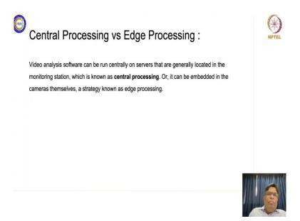
So, now we all know the difference between the central processing, versus the edge processing. And if we are trying to do it on the edge device itself, ok. So, for example, when you talk of video analysis software, it can be run centrally on the server that are located actually in the monitoring stations or data centers and this is called as central processing.
