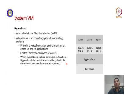
So, system VMs in detail so, that we can get some more idea about these stacks. So, basically the system VMs or system virtual machines are also called as hypervisors or
