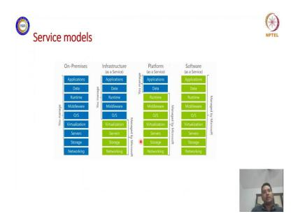
So, basically if you see from the different levels of the computing stacks. So, networking, storage, servers, virtualization layers, then operating system, middleware and runtime data and application. So, if you are operating on premise the entire stack of computing system. So, basically you have the entire server stack here and that is managed on premise then you have to manage everything.
