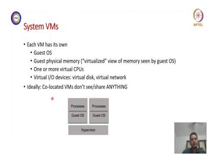
So, system level virtual machines we can see that each virtual machine has its own guest OS, own guest physical memory which is virtualized view of the memory seen by this guest OS. And, and let us say one or more virtual CPUs based on the allocation by the hypervisor and virtual IO devices which is abstracted by the hypervisor through this virtual machine. Now, ideally so, you can see that these two guest OSs can see or share
