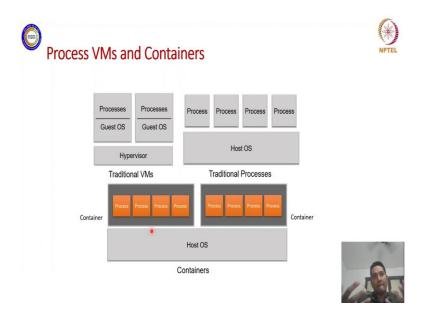
So, what we will do is that we will go in between of or the midway of these two extremes which is the container based approach. So, this is also one way of virtualizing things, but the thing is that here we are containerizing several processes which we think that these processes can talk to each other.
