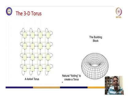
Or you start making these kind of toruses, here every box represents a switching element, every arrow represents the link between the switching element ok.
