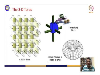
And then you keep on folding these connections and you create a very nice well defined mathematically explained topology. Therefore, you can actually put this equation into the routing engine of the switching element there which will now know where to send the incoming packet if it has a certain destination address.
