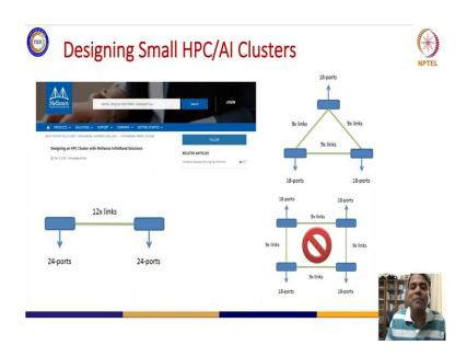
So, if you need to create a cluster ok, small cluster you will take multiple servers and you will let us say connect it all connect it all to that particular switch, the switch as you saw on the previous diagram contained around 40 ports.
