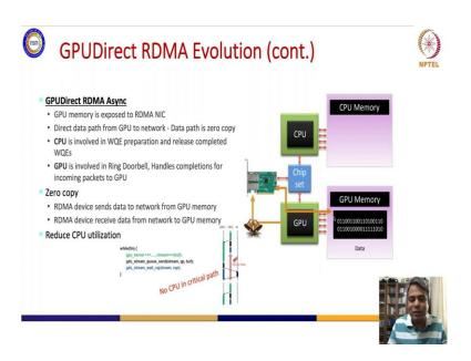
There are you know I talked about like there needs to be a control plane, which ensures that data corruption does not happen when two, three devices are simultaneously accessing or you know when to packetize and what to send, so there is a control plane. Earlier the control plane was actually controlled by the CPU, so and only the data plane was accelerated.
