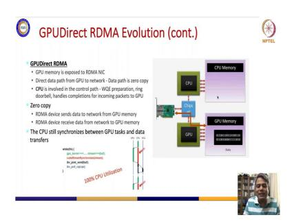
Why should I even copy it into the CPU memory, why cannot I have my network card directly access to GPU memory and therefore, save up all the cycles of sending data from GPU memory to CPU memory and this was also done.
