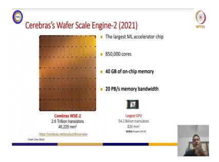
Now, one next generation of this wafer scale engine was published in 2021 and that has 850000 cores and that can deploy 40 GB of on chip memory and having a 20 petabytes per second of memory bandwidth. So, you can imagine how much the memory it is employed ok. So, just to have this shorter access time and reduced energy and. So, all these things we have seen in the previous slide right.
