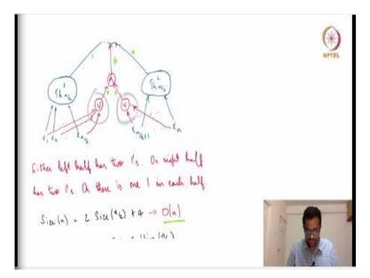
So, n divided by 2 times 4, so that leads to 2 n wires over here, then there are 5 wires so which I will mark with green, there is 1, there is 2, there is 3, there is 4, there is 5, there are 5 wires extra, so 2 n + 5. And then there are whatever wires are there inside each of these threshold n by 2 gates. So, 2 times wires of n by 2 which is basically the recursive called.
