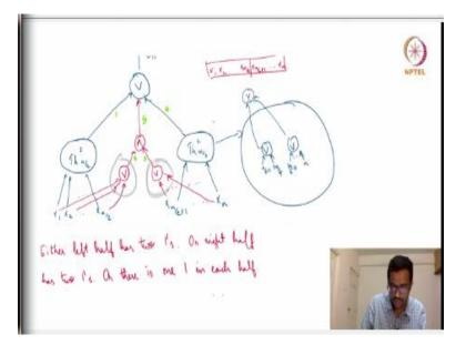
So, what I am saying is if you expand this threshold n by 2 gate, you will again find one OR gate that takes n by 2 + 1 to 3 n by 4, so I am expanding the right side threshold gate. And then another OR gate which has 3 n divided by 4 + 1 to X n, so I omitted the superscripts. So, it is X n by 2 + 1 to X 3 n by 4 and X 3 n by 4 + 1 to X n.
