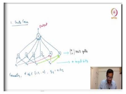
And if there are 2 ones in the input at least one of these AND gates will give us a 1. If there are 2 ones in the input X i and X j be the input, so there will be an AND gate with where which takes X i and X j as input and that will report a 1. And so we finally have an OR gate to check if is there any AND gate that is reporting a 1 or that is reporting true.
