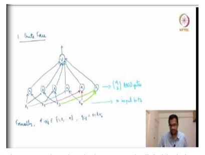
Again size and fan-in you may have heard when you study digital logic in your undergraduate. So, let us try to understand let us try to realize this function threshold 2 using some circuits. So, the first approach is what is the Brute force approach, so we are saying that out of the n bits input there are at least 2 ones. So, why not have a very simple idea? Try all possible pairs of in input bits.
