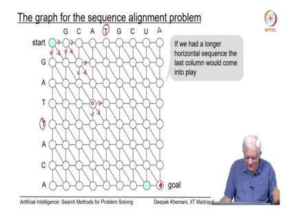
So, if you have let us say two strings in this example, the two strings are of equal length here. The one string is G C A T G C which is shown on the top. And the second string is G A T T A C A which is the which is shown on the left. And remember that the moves that you can make are either to the right or diagonally bottom towards the right or to the bottom.
