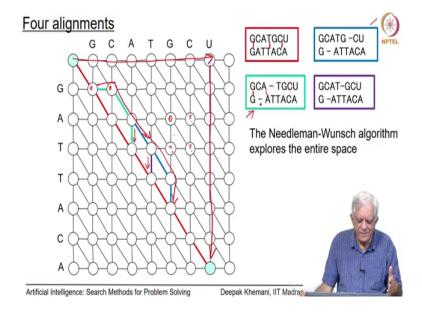
So, for these two given strings here are four possible alignments shown in 4 different colors. So, the first one is red which is simply saying that there are no gaps inserted. And as you can see the paths that this alignment represents is the diagonal from the start node to the goal node without any deviations in any place essentially.
