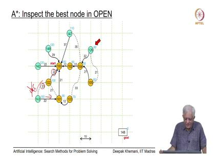
So, now it is going to expand this node with a f value of 104 and h value of 80 as before it generates that node which appears to be close to the goal node as before it picks that node and find that it does not make any headway in that direction and it shifts its attention back to a node which on the surface it looks to be in the wrong direction heuristic.
