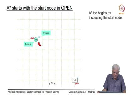
We start off with the start node as before and you can see that the label inside the node is 100 which is its f value. Remember its f value, but f value is equal to h value for the start node because g value is 0 because you are already at the you are already at the start node and this is the only node which is in contention. So, as all other algorithms algorithm A star also begins by picking this node as the first node for expansion.
