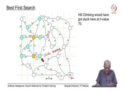
So, the next once it expands this node that it has just picked, its two neighbors you can see the one and the one here they will get added to the graph and now they have gone into the open list. So, the open lists are expanded we have more open nodes and the best looking open node is the one with the heuristic value 70.
