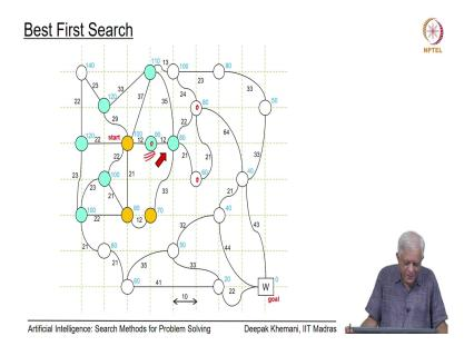
So, keep in mind that the nodes in orange or brown are the ones which have been inspected, the nodes in cyan are the ones which are the set of candidates or the open list and the best one is the one that is going to be expanded at each stage essentially.
