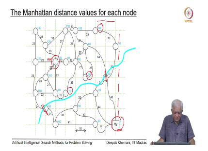
We will use a Manhattan distance for the sake of simplicity and further problem that we are trying to address here are the Manhattan distances shown in blue with every node. So, for example, this value has a value of 80. So, you can see that there are 2 segments here and 6 segments here and so, and since each segment is 10 units ok. So, this one is not there. So, these are the 6 segments. So, 6 plus 2, 8 and so, we have a distance of 80 essentially.
