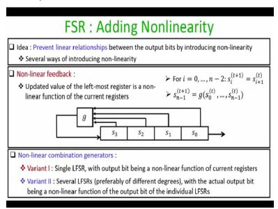
So a method which is used actually to preserve the security of the LFSR is to add some kind of non linearity. So if you see the attack, or the strategy, which is used by the attacker here is to explore the system of linear equation, or namely, the attacker uses the fact that the feedback is actually a linear function of the subset of the register. So one way to get around this is to add some kind of non linearity in the feedback shift register.
