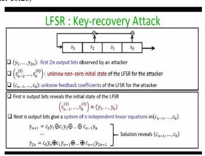
And adversary can recover the entire key and once it recovers, the entire key can recover or it can predict all the future output bits of LFSR right. So imagine you are given an LFSR of degree n where you do not know the feedback coefficients and you do not know the initial states of
