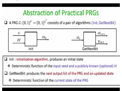
So in all the practical inst instantiations of pseudo random generators, we can follow the following extraction. So imagine you are given a pseudo random generator, which expands an input of little l bits to an output of big L bits right, we can assume that the pseudo random generator consists of a pair of algorithms, namely an initialization algorithm and GetNextBit algorithm. And what basically these algorithm does are as follows.
