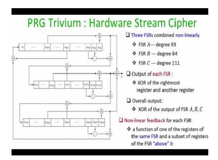
And it turns out that the modern constructions of PRGs based on LFSR are indeed used this principles. So here is a candidate construction based on LFSR, which is called trivium. And it is a highly popular instantiation of pseudo random generator. And it is basically if you see pictorially it is actually a combination of 3 feedback shift registers. So you have the first shift pack LFSR consisting of 93 register which we denote as the feedback shift register A.
