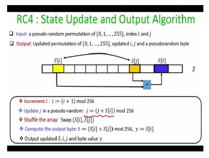
Now once the state has been initialized we actually now go to the state update and output algorithm. So, in each state update algorithm in each invocation of the state update algorithm, the current contents of the S will be shuffled around and one of the bytes is going to be output. So, the way it is generated then as follows. Imagine we have the current i and the current j, what we do is we increment the value of i.
