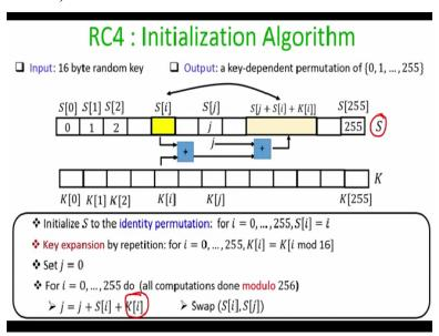
So now let us go into the details of the initialization algorithm. So the key or the key for the RC4 algorithm is basically a 16 byte key, which is going to be a random 16 byte key. So we denoted by k 0 to k 15. And output is going to be a pseudo random permutation of the set 0 to 255. So that is a array S. So we initialize the array S consist of values 0 to 255 in sequence, namely, we, the first byte is set to be 0.
