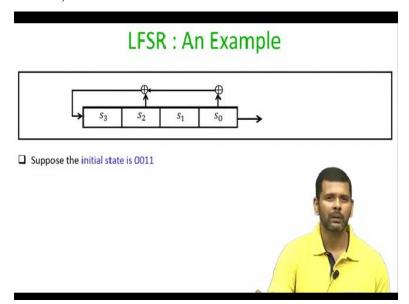
So for example, if you take this LFSR of degree 4, and suppose the initial state is 0011 right then after the first state doubt everything will be shifted by one petition and as a result, the bit 1 is going to be the first output bit and the feedback which will be going into the LFSR for the next iteration will be 1, namely the XOR of the bit 0 and 1 because your feedback coefficients 0101 and as a result the next state of the LFSR will be 1001.
