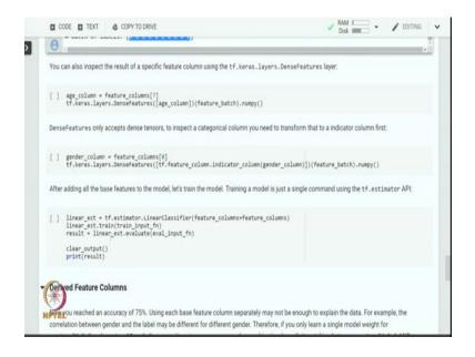
Let us define our logistic regression classifier using tf.estimator.LinearClassifier command. It takes feature columns as its argument, then we train the model by giving train\_input\_fn as an argument and we evaluate the model using eval\_input\_function as an argument. We get we store the result in the result variable and we will print it at the end of the execution.
