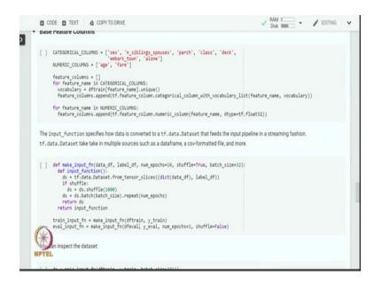
Then we define input function to specify how data is converted into tf.data.Dataset format that feeds the input pipeline in a streaming fashion. The dataset takes multiple sources such as dataframe, csv, formatted files and many more. Let us define a dataset from tensor slices and in if required shuffle the dataset and return the dataset in the batches.
