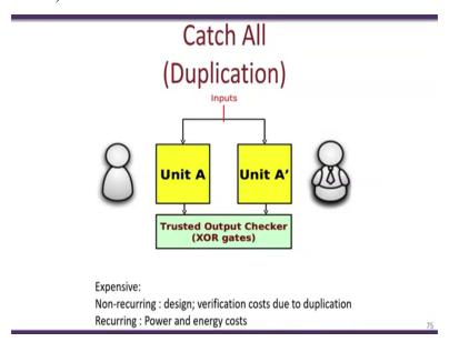
In such cases the worst case situation is where we could actually have two units possibly designed independently and both inputs are sent into both of these units and verified at the output. So for example we have a very complicated circuit over here let us say for example cryptographic algorithm and we want to ensure that this cryptographic algorithm does not have any Trojans.
