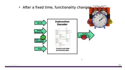
So let us start with trigger ticking time bombs. Essentially if we consider this as our hardware module what a ticking time bomb trigger does is that it waits for a fix time and then triggers the hardware Trojans payload to execute this time is typically specified by the attacker. The attacker we want that the Trojan's trigger gets activated may say after a few months a few weeks or maybe even a few years or maybe at a specific time during the year.
