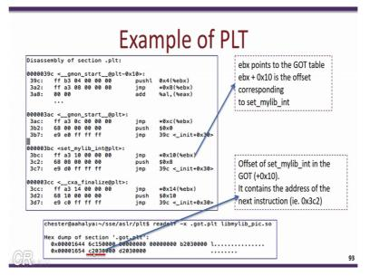
So let us dig a bit more deeper into the contents of setmylib\_int, so if you do a disassembly of this we see that setmylib\_int present at the location 3BC that is going to be in the PLT, so it
