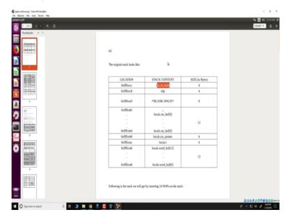
So what an ROP attack actually does, is that it replaces this return to main and starts filling in gadgets over here, so starting from the first gadgets which is placed at this point, you would have gadgets going upwards like this, such that each of these gadgets have some operation in computing the 10 factorial.
