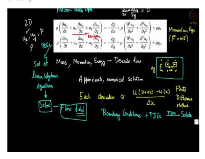
Okay, so suppose you want to predict this flow, what you do is apply an approximate numerical solution you cannot find exact solution, so you find out an approximate numerical solution and the way you do it is let us say each derivative for example the derivative here del u, del x you approximate it as u at x plus delta x minus u at x divided by delta x. Of course I am giving you a very simplified and simplistic example of how we do this.
