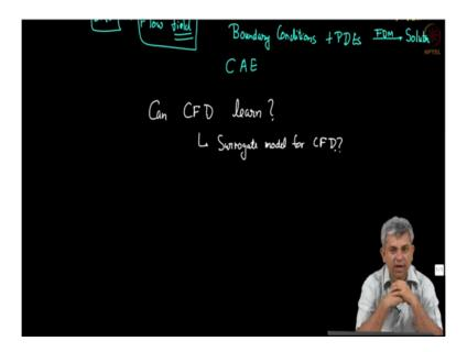
Now the problem with this is for complex bodies it can take you a very long time to actually solve these equations. So each time for example let us say I am doing a design of an aircraft or design of the shape of a car of a racing car, each time I make a small change in the shape of the body, I will have to go through a lot of computational time in order to get one solution.
