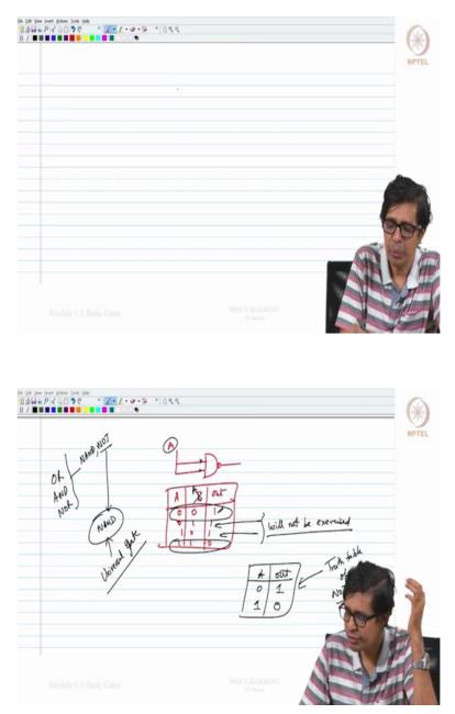
Now let us see suppose I connect to both the input of a NAND gate the same A what will be the output so we know that A B is out zero zero is one, zero one is one, one zero is one, one one is zero this is what the NAND gate this is how the NAND gate behaves this is the true table of the NAND gate now if I connect both the inputs to the same line that means only two of this four inputs are exercised this.
