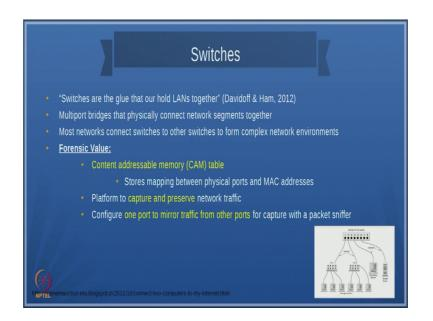
What switches, sometimes switches are also intelligent; that means, they learn the networks and some switches also throughout log information ok. Usually what happens is that if you see this diagram here switches combined two other switches and then that others which becomes very intelligent and essentially tries to learn where all the Mac addresses and all that, and routes the data based on the Mac addresses ok.
