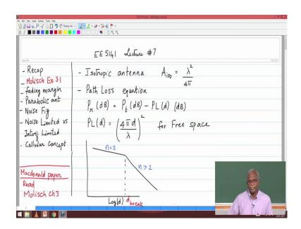
The one of the things that characterizes is the scale factors which we represent as the area of an isotropic antenna again it is a conceptual term basically it is something that is helpful for us in terms of the characterizing of the wireless link. So, the area of an isotropic antenna if we take it as a reference lambda squared by 4 pi, lambda being the wavelength of the carrier frequency then we derived 2 very important expressions.
