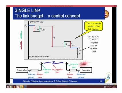
So, here is a simplified way of visualizing the link budget you have the transmitter that you can assume that as the output will be the power amplifier that gives you a signal at a certain level. Then you have the cables that connect you to the antenna that will cause a drop in the power because the that is the losses then the antenna gain it may boosted back to its original power or maybe boosted even beyond what the original power was that that is the level at which you transmit.
