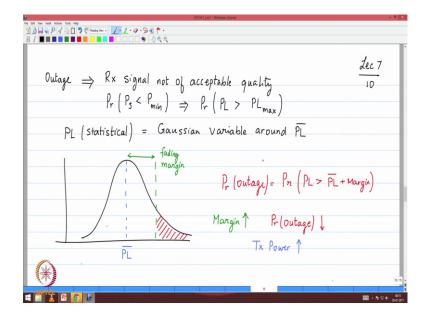
The; or you can think of it as average path loss average signal power is corresponds to average path loss as well. So, average path loss is what I expect to see, but there is a statistical variation and just for ease of visualization I have shown it as a Gaussian distribution around that in and very often it actually fits a model that is close to Gaussian. So, it is good for us to sort of use that as a baseline model.
