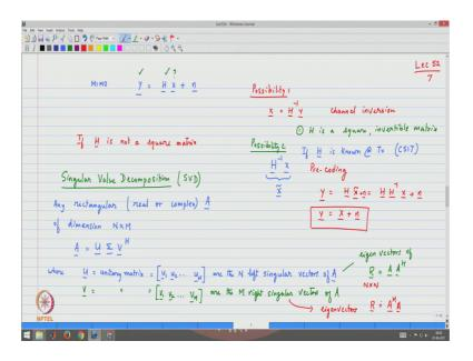
Now I would like to go back and re look at the equation that we have written down. So, the MIMO equation a MIMO system can be represented in terms of Y is equal H x plus n, and we are told that we are we have the observations of y and H is known, and we are trying to find out what is x.
