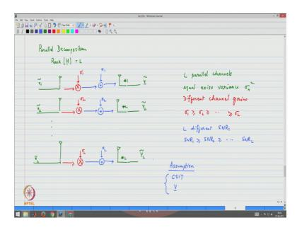
And I it I believe that gives us a lot of insight and what we would like to do is look at how we can represent this. So, the parallel decomposition of a MIMO channel parallel decomposition can be captured in the following form parallel decomposition. So, we have Nt transmit antennas and we have Nr transmit antennas, but effectively the number of channels the parallel channels that we have depends on the rank of the matrix.
