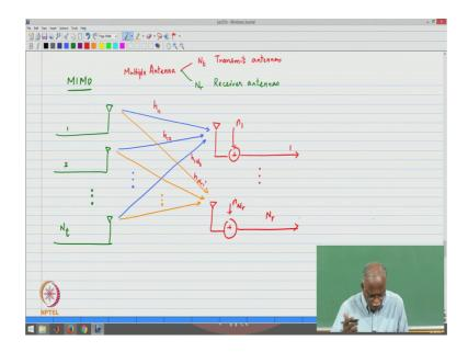
So, with that in mind we would now like to look at the formulation of the multiple antenna environment. So, multiple antennas at the multiple antennas and transmitter receiver which it is been characterized in terms of there are Nt transmit antennas. So, Nt antennas at the transmit and transmitter and correspondingly we have Nr antennas at the receiver. So, Nr receiver antennas.
