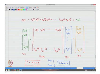
So, if you were to write down the output of the at the receive antennas y 1 of n, which is the first receive antenna this would be h11 of n times x of n x 1 of n the first transmit signal from the first transmit antenna, then h 12 from the h 12 of n n basically shows that these are all time varying quantities the channel can be a time varying quantity.
