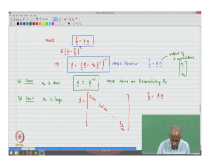
We say that b hat will be equal to A times r, and we wanted to minimize b minus b hat magnitude squared expected value, and this resulted in us obtaining the matrix A in the following manner which is R the correlation between the spreading waveforms plus N naught that is the noise variance of each of the antennas multiplied by D inverse and the whole inverse.
