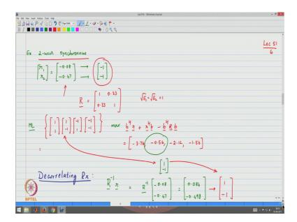
So, we have looked at the following example I would like us to quickly look at it once more it is a two users synchronous CDMA, at the receiver the values of the output of the first correlator and the second correlator are given by minus 0.08 and minus 0.47.
