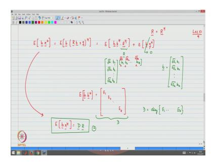
Now, please write down or substitute the value for r, this would be expected value of b times R b plus eta Hermitian and this would be equal to if you were to expand it, it would be equal to b times b Hermitian times R Hermitian, but we know from the property of the auto correlation matrix that R is a has satisfies the property that R is equal to R Hermitian. So, we could equivalently write this as instead of R Hermitian we could write it as R.
