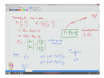
Now on the other hand the decorrelating receiver was formulated differently. So, if the received vector not the received continuous time wave form, but this is the vector of outputs this is the outputs of the k correlators, and if you write down the expression for that the output of the k correlators comes out to be r which is the correlation matrix which takes into account the correlation between the different spreading waveforms.
