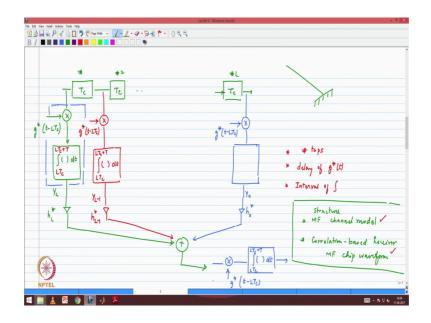
So, that is the summary of the rake receiver basically this is the form that we had looked at there are L plus 1, L plus 1 taps and basically each of those taps gave us a went through correlation based receiver which is multiplied by g star and then followed by integration then the corresponding coefficient added together.
