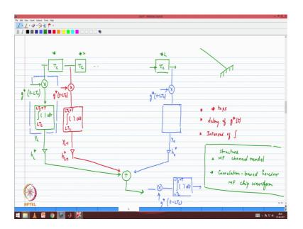
So, the structure is a tapped delay line with L delays; L delays of T c each of these branches keep in mind is being multiplied by g star of t minus L T c t minus L T c means g star of t delayed by L T c and then it is being integrated because I delayed g star by L T c. My integration limit starts from L T c to L T c plus t. Now of course, we showed that we can rewrite this as 0 to t and keeping j star of t not the shifted version. So, if you keep
