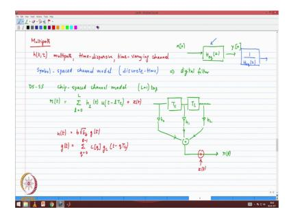
So, let us quickly set up the framework for multipath and then see how to. So, we have a time varying time dispersive channel no problem we know how to characterize that. So, we will describe this as a multipath time dispersive time varying channel remember we have the three dimensional graph which we draw and. So, this is not this is very familiar to us time dispersive time varying channel that is represented by h of t comma tau, t is the time variation tau is the delay dimension ok.
