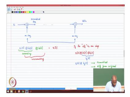
So, now how does the scrambling work if I have a input information sequence si binary, I can do a modulo 2 addition with my m sequence which is also represented in the binary form modulo 2 addition, and this will come out to be a scrambled sequence, ok.
