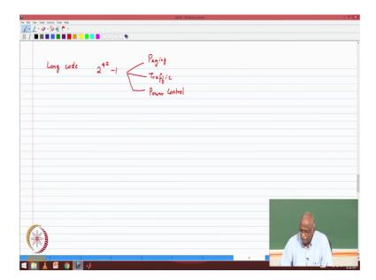
What about the I said there are 2 codes, one is the short code the other one is the long code. The long code consists of a 42 shift register 2 power 42 minus 1, this is used in the paging channel to scramble it is also used in the traffic channel with a user specific mass. So, it is not just the m sequences some additional modification and this is also used to tell you where to insert the power control bits.
