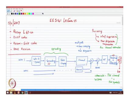
So, for user 1 you would have the information bits, this is user 1 and you would map it on to a symbol that would be exactly as you would do for a narrowband system bits to symbol mapping depending upon what the constellation modulation using, we have been looking at the binary as a simple form, but you do not have to limit yourself.
