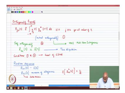
The 2 properties that are very important for us, one is mutual orthogonality that makes me robust against other users codes and self orthogonality and both of these are necessary for us to build a CDMA system. So, maybe just to reemphasize the mutual orthogonality is what helps me be robust against multi user interference. The common
