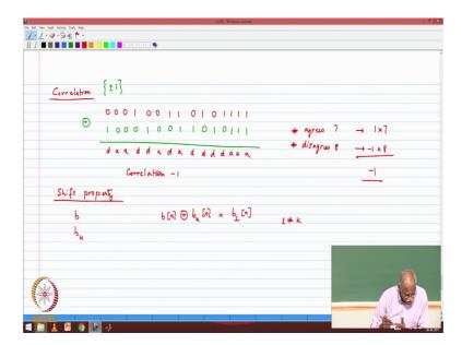
I would like you to do the following correlation. The correlation is between the basic sequence and sequence that is right shifted by one. So, the basic sequence is  $0\ 0\ 1\ 0\ 1$  0 1 0 1 1 1 like get at a 1 1 more 1 is that. So, now, do a circular shift. So, the 1 comes to this time then come  $0\ 0\ 1\ 0\ 1\ 1\ 1\ 0\ 1\ 1\ 1$  ok.
