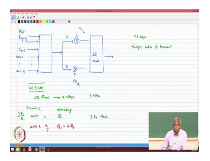
Now, I have the base station signal, I have paging that is going in then there is the before paging even the pilot is going in, there is the sink channel that is going in, and then I have a whole bunch of users. So, it could be user 1 to user n all their signals basically you know using different codes all of them punctured power control all of that is and I come out with date of sequence and the same data is sent on both the I and the Q
