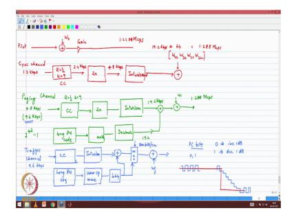
So, the pilot channel is all zeros on it you superimpose the w 0 which is also all zeros, and then you apply some gain to it you want to you may want to boost the pilot channels you can have good channel estimation. So, that is your first one that is your I am sorry this is this is pilot channel. So, this is pilot. The second one is sync channel, sync channel this is how it is transmitted in CDMA 2000, the sync channel it does not have very high data rate its 1.2 k b p s is the information rate.
