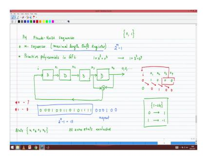
So, in the shift register sequences, if you think of x 1, x 2, x 3, x 4 as a state x 1, x 2, x 3 x 4 as a form of a state of the state machine, then it will cycle through the maximum length shift register sequence basically says that the this interconnection is such that the state we will not repeat until you have gone 2 the power of m minus 1, why is it m minus 1 because the all 0 state is excluded, because once you go into the all 0 state you will not come out of it.
