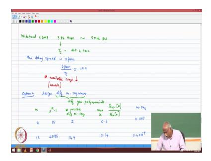
So, the wideband CDMA system I will already start to introduce these numbers so that you will become familiar with it before we actually come to that. Wideband CDMA system uses a spreading factor or you know the spread bandwidth is 3.84 mega chips per second MCPS so; that means, the bandwidth of the signal will be 3 around 5 mega hertz.
