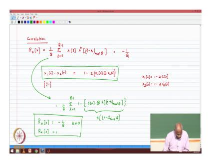
So, basically if I now define a correlation I am defining a very specific type of correlation is not the definition R x of k is defined as 1 over Q, summation l is equal to 0 through Q minus 1, x of l, x star of l minus k modulo Q. Modulo Q means it is a cyclic shift basically. So, what this says is I am I have defined my autocorrelation in terms of a sequence with cyclic shifts of itself.
