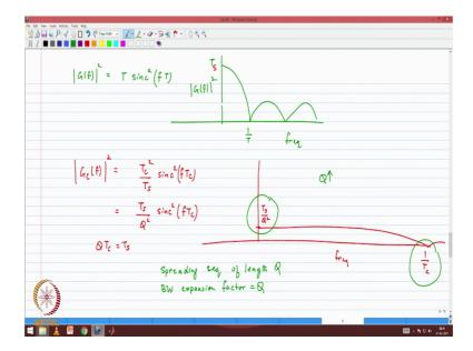
So, now what we have on before us is the following if it was a conventional modulations scheme the spectrum that we achieved or the g of f magnitude square we wrote down was t times Sinc square f t. So, basically it would it is a Sinc function starts at t this is a 1; 1 over t as the first point at which the; so, this is frequency; this is mod g of f square.
