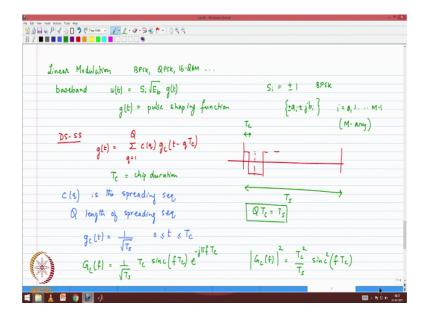
So, if it was not a spread spectrum system just a regular digital communication system with linear modulation linear modulation. So, linear modulation can be BPSK can be a QPSK 16 QAM all of these are linear modulation methods dot, dot, dot the baseband signal; baseband signal representation will be u of t will be the complex signal let me call that as si scaled for energy purposes root e b whatever is the e b that you want to achieve multiplied by the pulse shape g of t.
