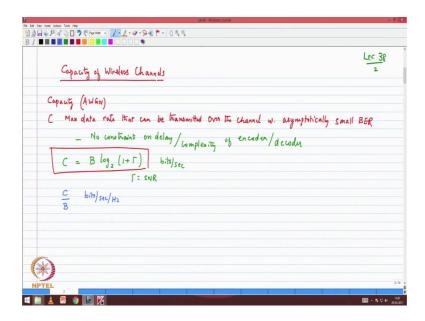
So, hopefully this will be a interesting lecture. A very quick run through we are having as the foundation Shannon's definition of the capacity of a AWGN channel B times logarithm base 2 1 plus gamma is the SNR and the units are bit is per second. So, this is
