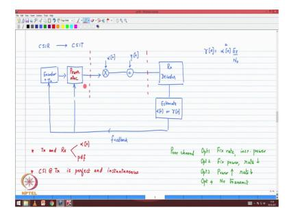
So, the context of CSIT is as follows, we have the channel as before a fading channel. Fading coefficient plus AWGN have to design the encoder and decoder the only difference is now is that I can estimate SNR and I can feed it back. I can feed it back for 2 purposes one is one is to choose encoder decoder, but more than that to also do power allocation because now I can do differential allocation of power for the different channel realizations.
