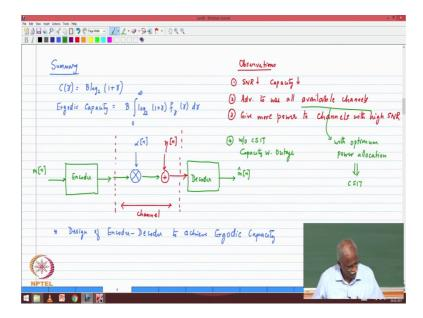
That this capacity is for these specific scenarios with in terms of SNRs and the probabilities of the different SNRs, and using the Jensen inequality we showed that the ergodic capacity will always be upper bounded by the corresponding AWGN capacity ok.
