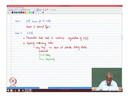
So, now, we let us go little bit deeper just to sort of quickly run through, the 3 cases are when I know only the PDF then the when the channel receiver knows the channel state information, and the way we would achieve a capacity in this case is to have very long code words. Again we talked about the delay and the complexity of such systems.
