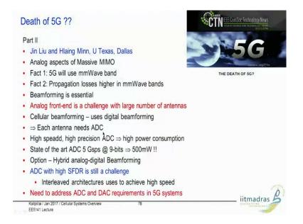
Let us say you want to transmit at 100 megabits per second, then the caution is that today's ADCs that have to run at such high powers such high speeds with resolution of 9 bits or 12 bits will consume a lot of power. So, for example, today's state of the art a to d converter at 5 giga samples per second 9 bits precision actually consumes 500 milliwatts that is a lot of power if you have now 64 of them running in a device you know it will be very very power hungry.
