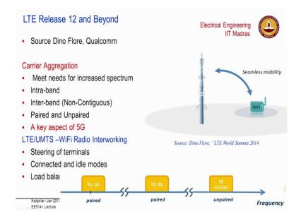
The spectrum that is available today in the 2G and 3G is scattered in different frequency bands 800 band, 1900 band and in the 22.3 gigahertz band. The aggregation of a carriers. So, typically if you want 10 megahertz you like to have it all 10 megahertz together contiguous, but if you do not have 10 megahertz contiguous can you aggregate carriers from different frequency bands and that is also being talked about.
