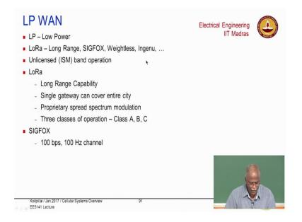
LP is low power and again these are devices that are optimized for very low power, a LoRa is long range combined with low power and a Sigfox is actually low rate combined with the with low power.
