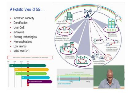
So, a holistic view of 5G, we have to address increased capacity that is number one, a densification will happen how much we have to see it has to be done in a controlled manner. Millimeter waves will be introduced because we want more spectrum and very very important we are looking at a lot of machine type communications which have low latency and high reliability.
